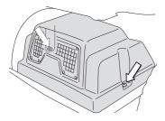
2 Rider 213 C, Rider 216 Check that there is oil in the transmission's oil tank. Fill if necessary with engine oil SAE 10W/40 (class SF–CC).
